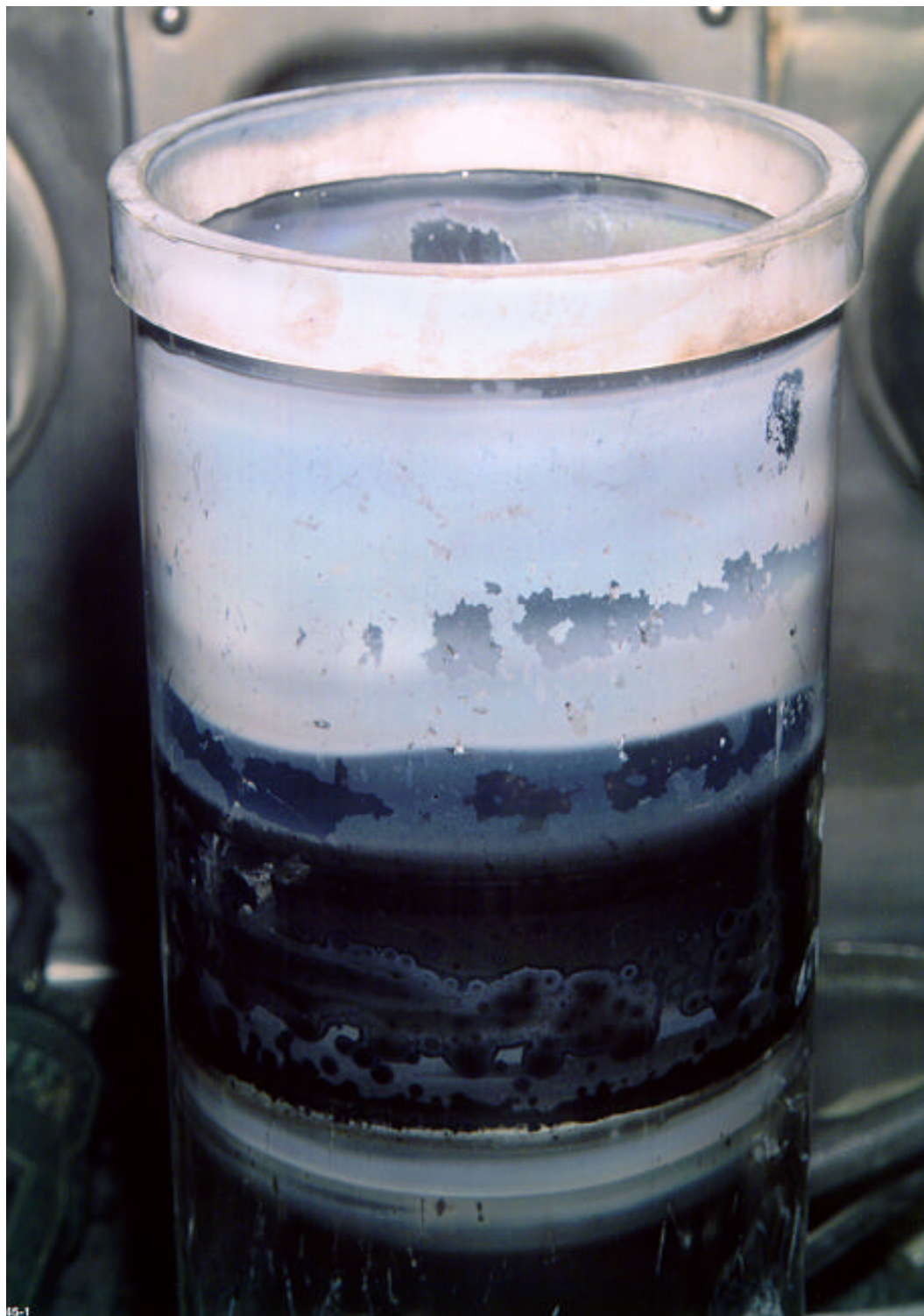
Figure 7b. Top-half of Vycor tube used for vacuum containment of standard plutonium casting furnace after a single casting of a poor electrorefined ring into rods.
